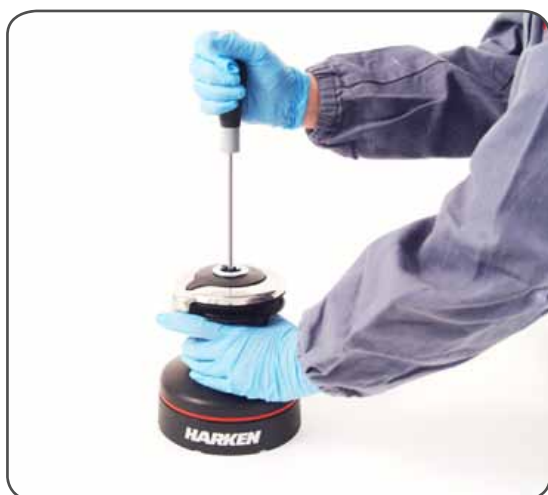
1. Unscrew the central screw ( \approx 2\text{Nm}/18\text{ in-lb} )
