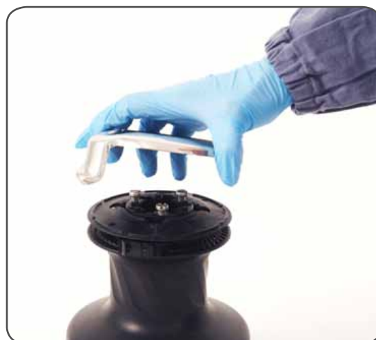
4. Remove the stripper arm n°27 by rotating and lifting it.
