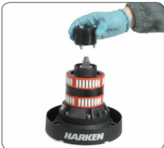
6. Completely unscrew the three screws n° 28 and remove the stripper arm support n°22
