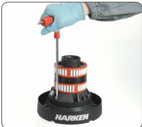
6. Completely unscrew the three screws n° 28 and remove the stripper arm support n°22
